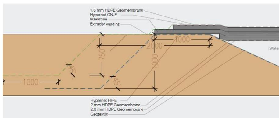
*Fig. 8: Cross section of the edge of the floating cover (Vang Jensen 2014)*
