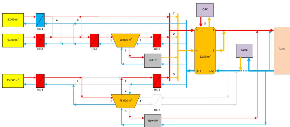
**Fig. 6:** Function diagram for the TRNSYS model of the production plant in Marstal (PlanEnergi Deliverable 2.1, March 2013)
