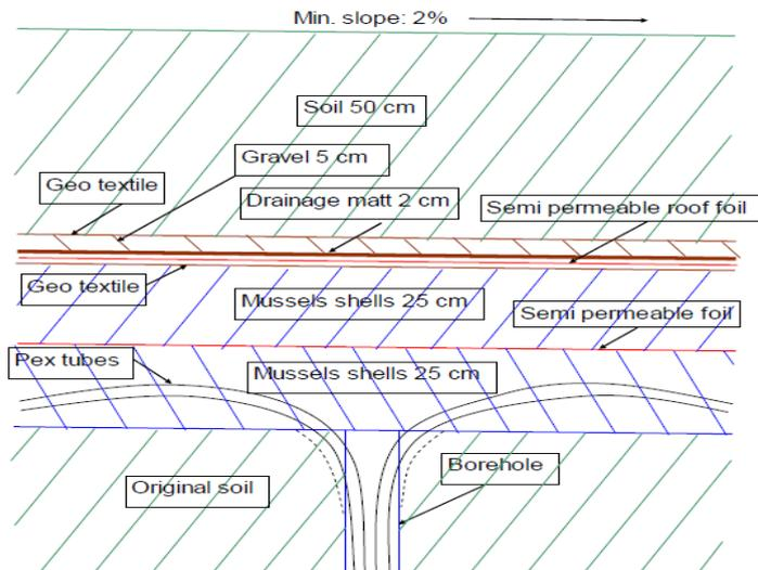
*Fig. 3: Section view of the cover indicating the layers of the construction (Sørensen et. al 2013).*
