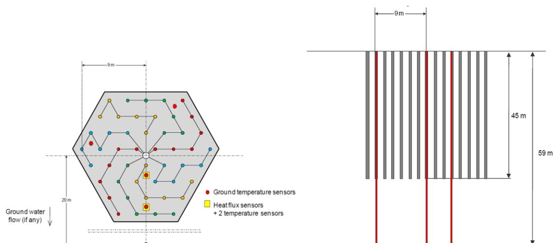
Fig. 2: Layout of the BTES in Brødstrup, top view and cross sectional view (Sørensen et. al 2013)
